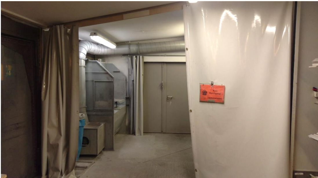
Figure 34: Spray booth at Innovint. The curtain on the left- and right-hand side is closed before the paint job starts
