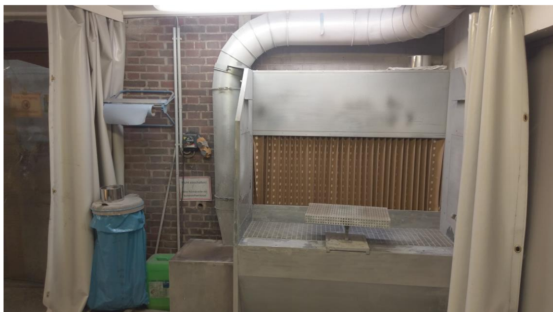
Figure 35: Spray booth at Innovint: shown is the extraction system, wherein parts are painted.
