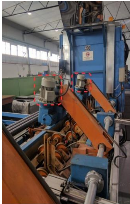
Figure 53: Vibration Sensors on KLEEMANN's Polishing Machine
