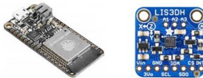
Figure 50: SP32 board and Lis3DH on a breakout board
