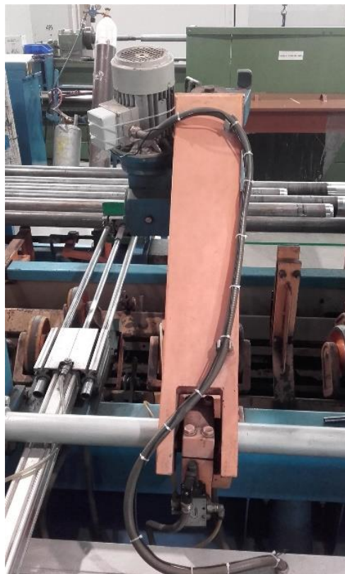
Figure 52: Installed sensor on the polishing machine
